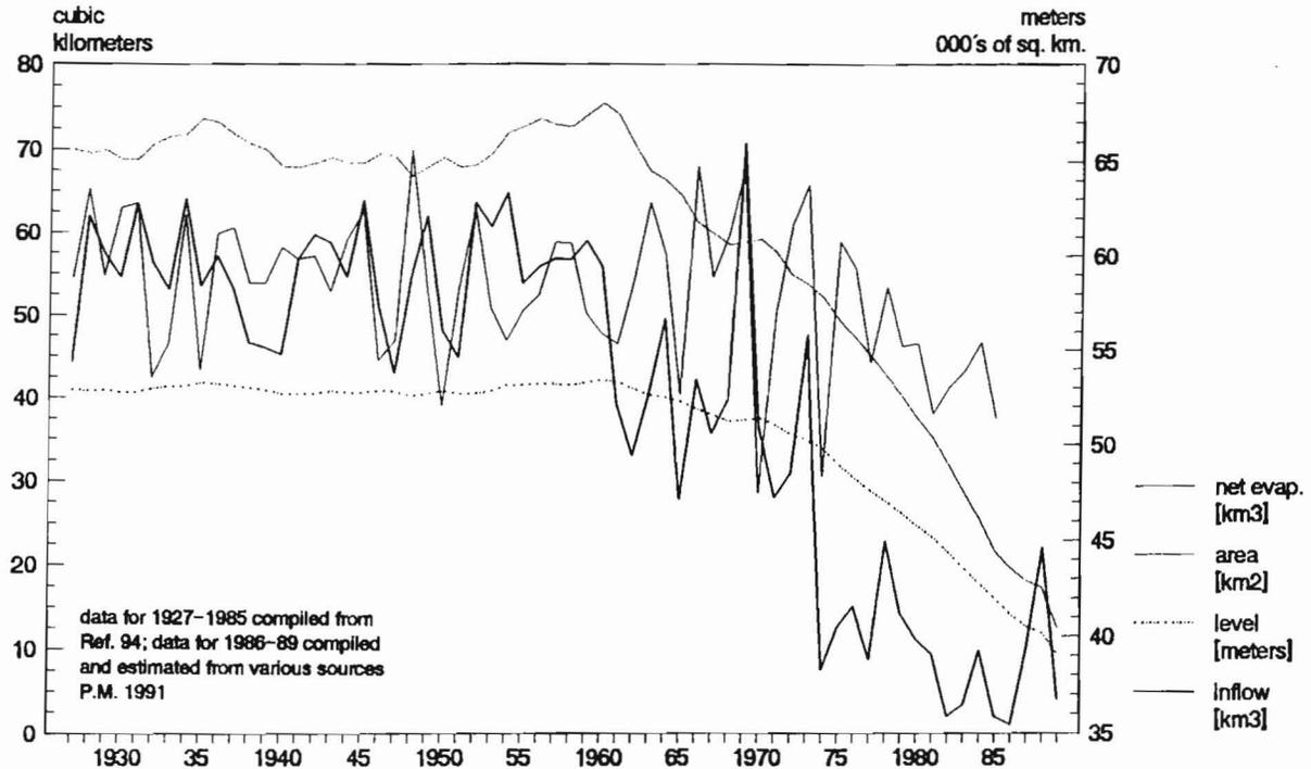
Figure 6. Water Balance Parameters of the Aral Sea, 1927-1989
